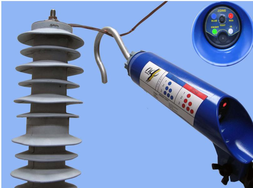
Arrester test with the ADD™
